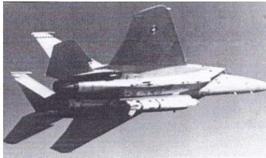
Fig. 4. ASAT anti-satellite missile system with F-15A carrier aircraft
